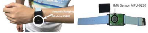
Fig. 8: WearCoach prototype. A ultrasonic distance measuring module KS102 and an IMU sensor MPU-9250 are used.
